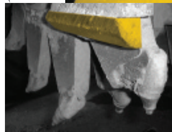
KenCast on a side cleaner bar of a reclamation machine.
